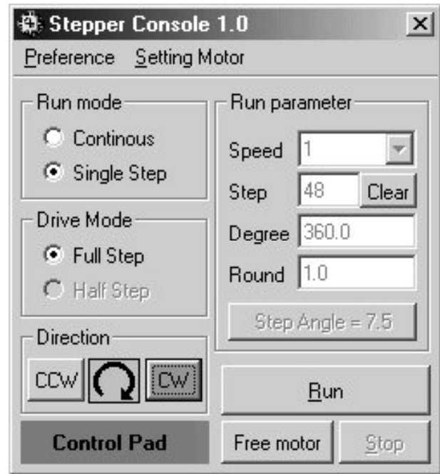
Figure 7 shows the example setting about selection motor rotate in single-step mode.
