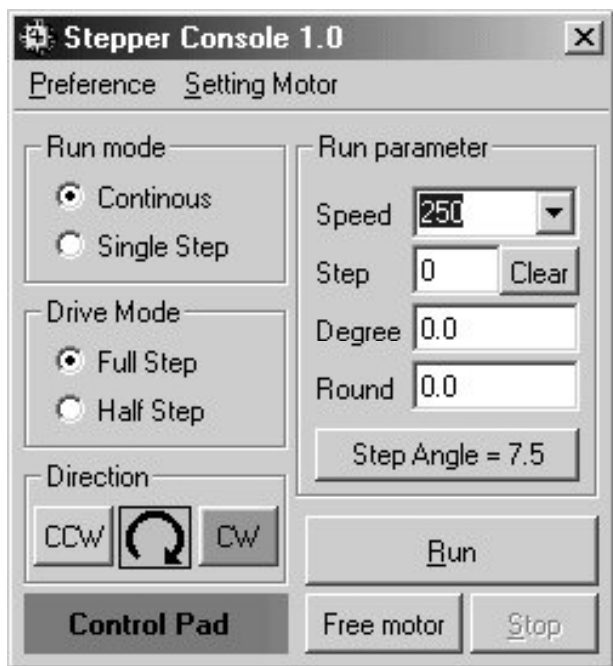
Figure 4 The example setting about set the motor rotate continuous in clock wise direction with full step mode at maximum speed and step angle of motor is 7.5 degree/step.
