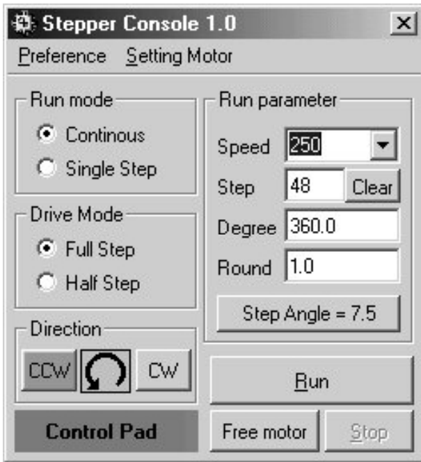
Figure 6 shows the example setting about selection motor rotate in counter clock wise direction, full step mode, step value 48 steps to stop.
