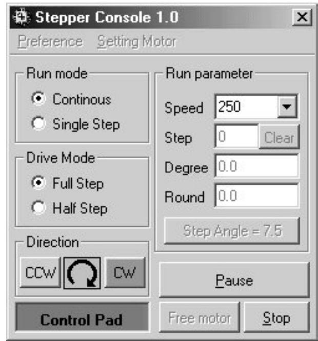
Figure 5 The operation window after click Run button in Setting window from figure 4.
