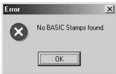
Figure A1-9 shows Error box on screen. It means software cannot detect i-Stamp. Must back to check serial port cable again and check FREE serial port
